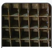
Grid is difficult to clean. A dirty evaporator can cause diminished production, increased service cost and premature equipment failure.
