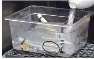
\* Remove retainer rod (take care not to bend excessively) from bottom of the float switch housing & clean all float parts.
