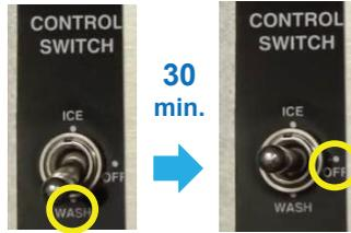
9 After **30 minutes**, remove **Front Panel**, then move the control switch to **OFF**.
