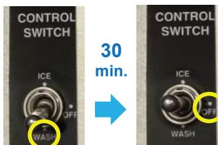
**⚠ NOTICE! DO NOT** leave the control switch on **WASH** for extended periods when water tank is empty. It will damage water pump seals.
