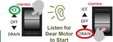
**i** The icemaker might make a noise/squealing when first started due to scale removal from auger/evaporator. This is normal in bad water conditions and will subside after 20 minutes.
