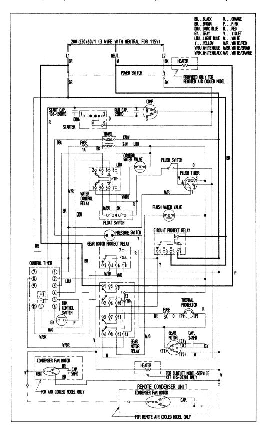
[g] When Flush Switch is moved to "FLUSH" position, Flush Water Valve opens and flushes Reservoir and Evaporator.
