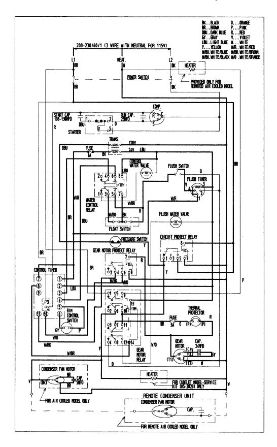
[c] Compressor starts about 60 sec. after Gear Motor starts.
