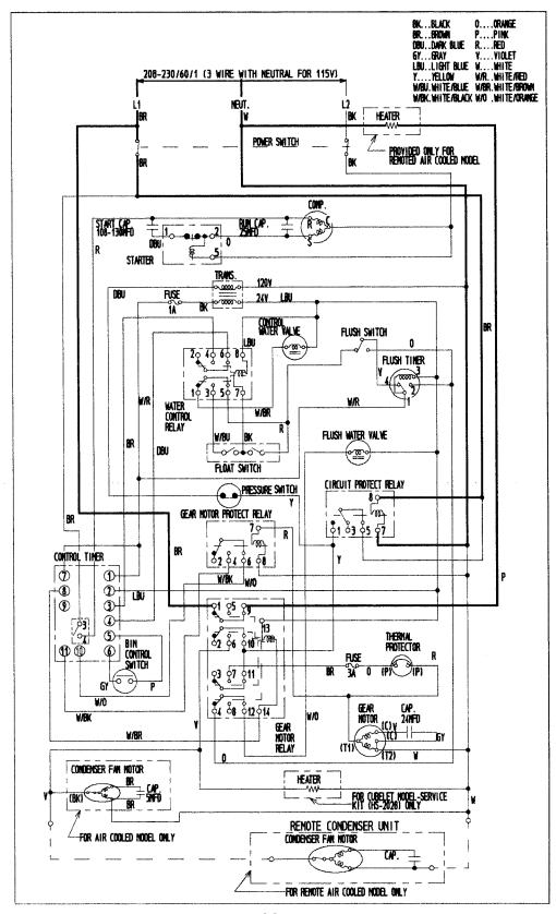
[j] If Gear Motor Fuse (3A) blows, the Compressor and Gear Motor will turn off immediately.
