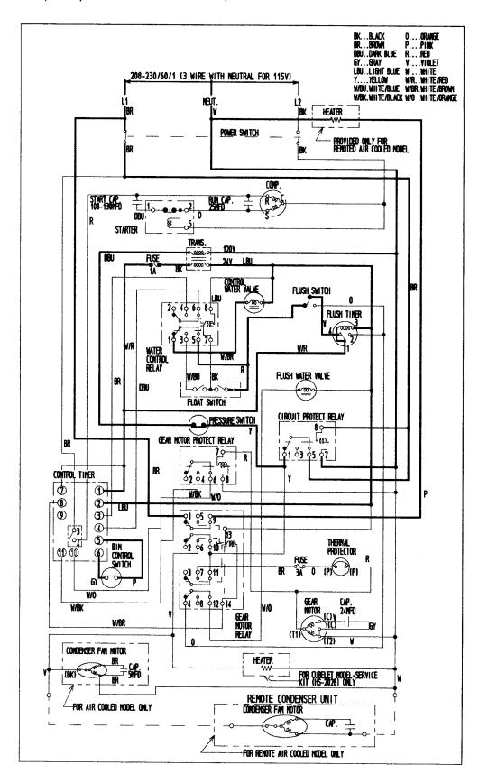
[f] Low Water (Water-cooled Model), or Dirty Air Filter (Air-cooled Model), Pressure Switch to "OPEN", Compressor and Gear Motor operates intermittently.
