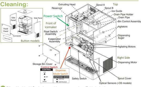
Dilute Hoshizaki Scale Away with warm water (see Table below). Remove the Storage Bin Cover<sup>†</sup>, Spout B, then Spout A. Pour cleaning solution into the Extruding Head until the Evaporator Assembly and the Reservoir are full and the solution overflows into the Drain Pan. Replace Spout A & B, and the Storage Bin Cover. Allow the icemaker to soak for <u>10 minutes</u>. <sup>†</sup>Use a 15mm socket to easily remove thumb screws.
